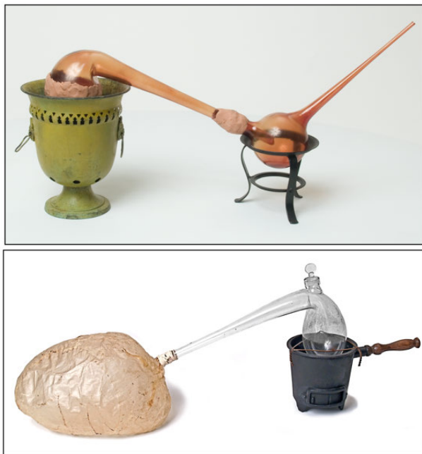
Figure 11. Top : Reproduction of an 18th-century, brown-glass retort with luting, quilled receiver, and charcoal furnace. Bottom : Reproduction of an 18th-century tubulated retort, gas bladder, and charcoal furnace similar to those used by Scheele.
