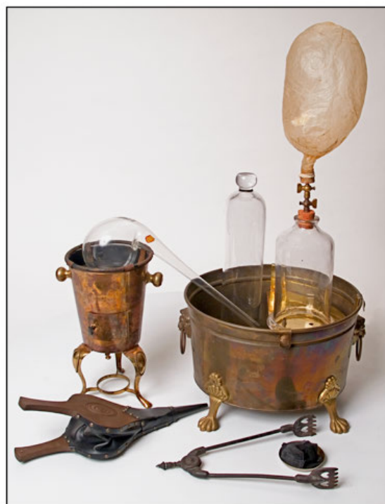
Figure 10. Reproduction of an 18th-century retort, pneumatic trough, and charcoal furnace similar to those used by Lavoisier.
